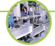
**ELECTRON GUN** Bursts of electrons are injected into an ultra-high vacuum stainless steel tube.
