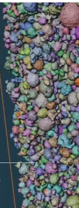
Computed tomography image of a Li-ion battery electrode material
