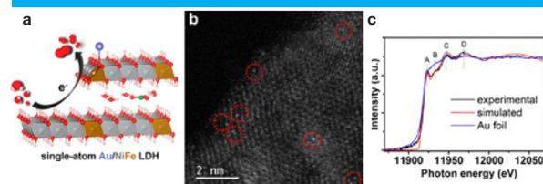
Figure 1 A) Two-layer DFT slab model for the <sup>197</sup>Au/NiFe LDH with interlayer CO<sub>3</sub><sup>2-</sup> anions and water molecules; B) HAADF-STEM; C) Comparison of Au L<sub>3</sub>-edge XANES of <sup>197</sup>Au/NiFe LDH, Au foil, and DFT guided theoretical modeling.
