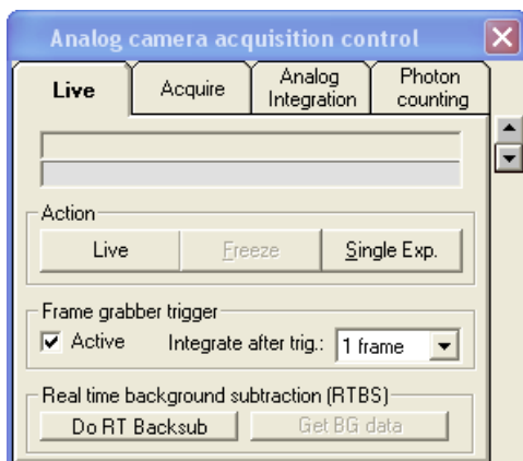
Fig. 23: The “Analog Camera acquisition control” window showing the most common configuration. The number of frames may need to be changed depending of the horizontal sweep (see 3.11.2).
