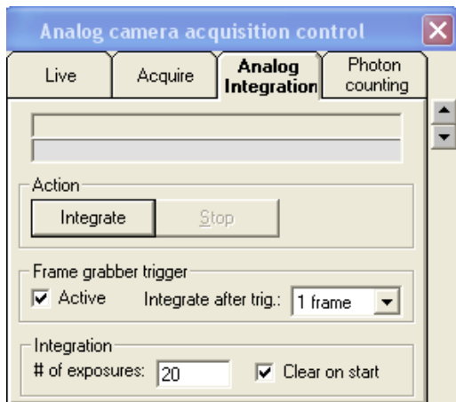
Fig. 31: The “ Analog Integration ” settings in the “ Analog camera acquisition control ” window.
