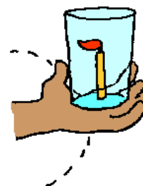
A candle flame accelerometer indicates an inward acceleration
