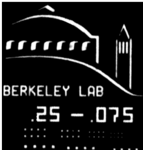
Figure 10-7 Resolution demonstration using two test patterns (electron-beam-generated patterns in gold deposited on silicon nitride). The star test pattern shows the diffraction-limited resolution predicted for the zone plate (35 nm outer zones, 150 \mu\text{m} wide). Zone plate and test patterns were prepared by Erik Anderson et al. (CXRO, LBNL).
