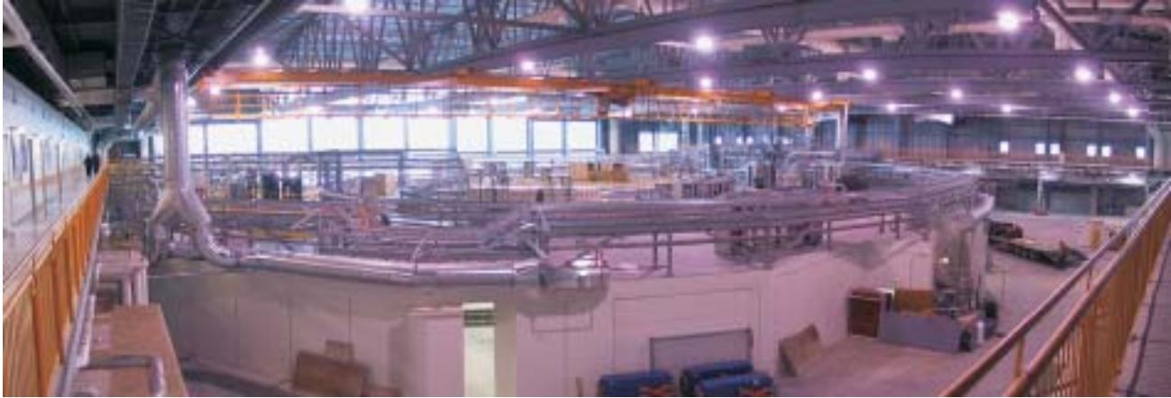
Panoramic view of the shielding tunnels of the CLS storage ring and booster ring (November, 2001).
