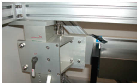
Figure 3 A front view of the left tower support structure showing the wire/pulley system and anchor shackle/eyebolt that can be used to raise or lower the main LTP beam. Also visible are the precision drilled holes in the tower (15 mm spacing over a range of 510 mm) to which the height can be adjusted, and the lever/expanding pin that is used to align and level both sides to better than 1 mrad, before lock-down.
